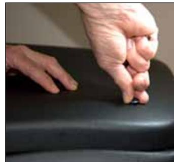
7. Avoid cross threading the screws by starting them by hand. You may need to locate the screw holes with a thin screwdriver to align them.
