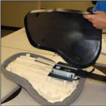
1. Remove the back from the chair and back outer. (Refer to *Back Outer Replacement* sheet.)
