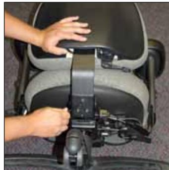
10. Reinstall back on chair, using the same three 3/16" Allen-head screws you removed in Step #1.
