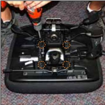
5. Remove the mechanism from the seat pan by removing the 4 screws (or bolts depending on the model). Use a screw driver if the seat is a 4, 5 or 7 which was manufactured after Sept. 1998 or a 6 manufactured after Apr. 2000. If your chair has been manufactured before Sept. 1998, the seat is held in place with nuts and washers and will require a 7/16" deep socket and ratchet. If not, use a 3/8 socket.
