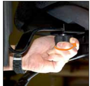
8. Reinstall the hand wheel with washers in place (lock-washer on first, then beveled washer with concave side down) and tighten at desired width setting.
