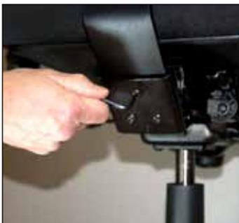
9. Secure back onto chair using the same 3/16" Allen screws from Step 1.
