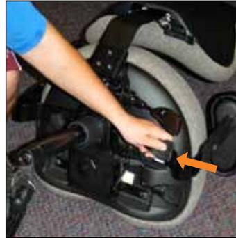
3. Extend cylinder to full length using seat height lever. Slide cylinder cover fully away from the chair so its out of the way.
