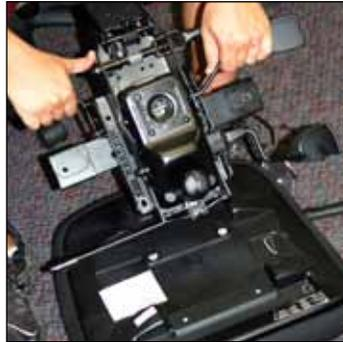
6. Lift the mechanism off the seat pan from the rear.
