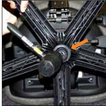
2. Wearing safety glasses, hold one leg of the base (gloved hand recommend) and strike the cylinder protruding through the base, using a plastic or rubber hammer in your other hand. The force will dislodge the base.\*
