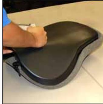
3. While lifting on the shell, apply a downward force with the other hand on the outer edge of the shell to release internal tabs.
