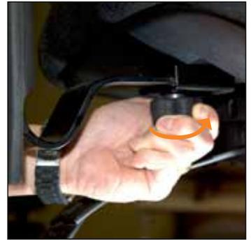
4. Reinstall the hand wheel with washers in place (lock-washer on first, then beveled washer with concave side down) and tighten at your desired width setting.
