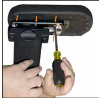
1. To tighten the resistance/friction of the tracker piece, tighten the 6 Phillips-head screws located along the bottom of the tracker piece. You may need to slide the tracker to gain access to the middle screws.
