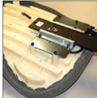
7. Replace with new assembly and install with the 4 screws previously removed.
