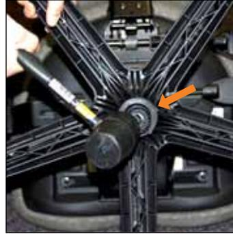
3. Remove the base according to instructions (Refer to *Base Replacement* sheet.)
