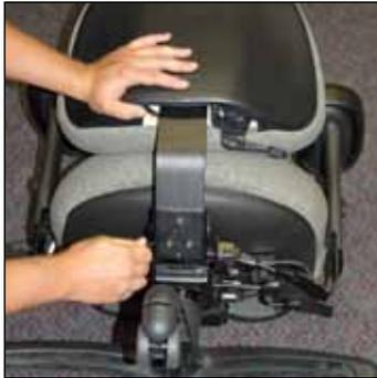
1. Remove the 3 screws (3/16" Allen-head) that secure backrest post to the mechanism.
