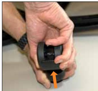
2. Holding base, grasp and pull the caster or glide straight up and out of the base. If any are stuck, you can pry it out using a flat screwdriver.
