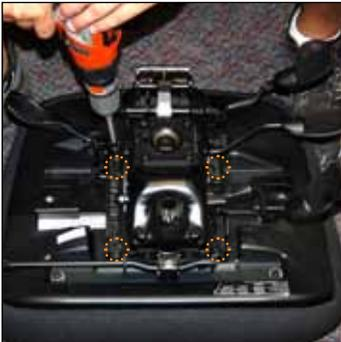
5. Remove the four 3/16" hex-head bolts (or nuts depending on the model) that secure the seat to the mech. **IMPORTANT:** Take note of any spacers that are positioned between seat and mechanism, as they must be in place on new mech installation.
