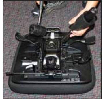
4. Remove the cylinder from the mechanism by firmly grasping in one hand and using a hammer to tap on the flat surface of the mechanism close to where the cylinder is joined to the mechanism until it comes apart.\*\* This may take several blows.
