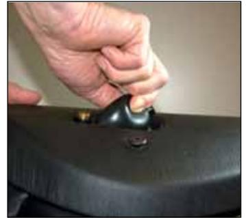
4. Pull the air hose from the nipple of the air bulb. Remove the bulb from the outer shell and reinstall into the replacement outer shell.
