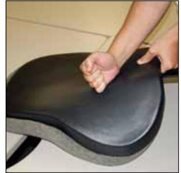
4. Repeat the previous step on the opposite side of the shell. If tabs break, remove the broken pieces from the back.
