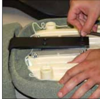
2. Remove the four 5/32" Allen-head screws that secure the headrest bar to the internal height adjuster. Remove the old headrest and place the replacement headrest in the same position for attachment.
