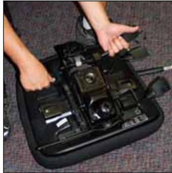
7. Replace with the new mechanism and attach to the seat by inserting screws previously removed.
