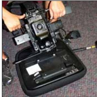
6. Lift the mechanism off the seat from the rear.
