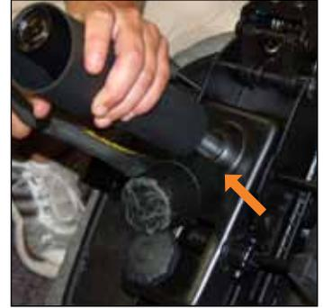
4. Remove the cylinder according to instructions (Refer to *Cylinder/Telescoping Cover Replacement* sheet.)
