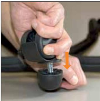
5. Install casters into new base with downward pressure until each is snapped securely in position.
