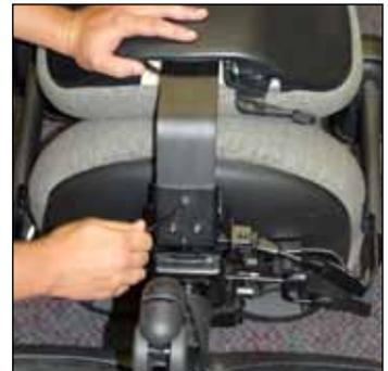
8. With new back shell attached, reattach the back assembly with 3/16" Allen-head screws in reverse steps from Step 1 above.
