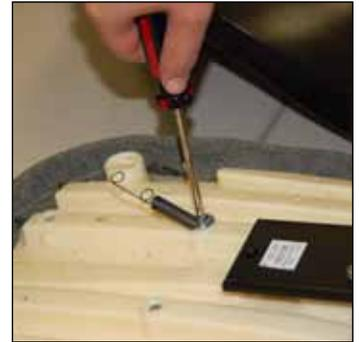
4. Using a Phillips screwdriver, remove the screw and washer holding the opposite end of the spring.
