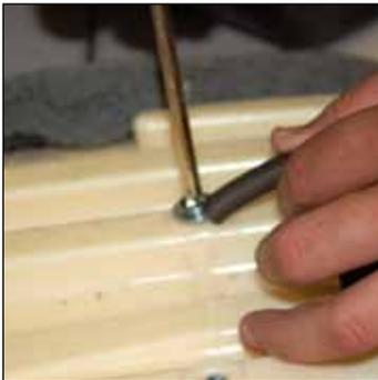
5. Insert the screw with washer into keeper ring of the new spring and reattach to the back in the same hole.
