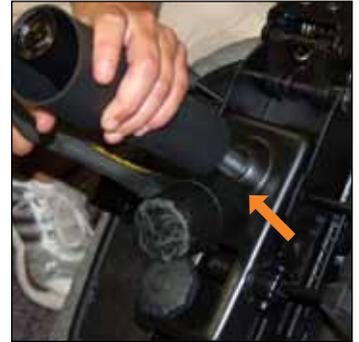
4. Firmly holding the cylinder with one hand, use hammer to strike the mechanism around the cylinder entry point.\*\* Several strong blows may be required to dislodge the cylinder from the mechanism.
