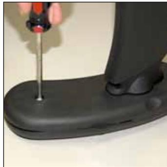
6. Secure the new pad to the arm assembly using the same screws you removed earlier, in Step 3.
