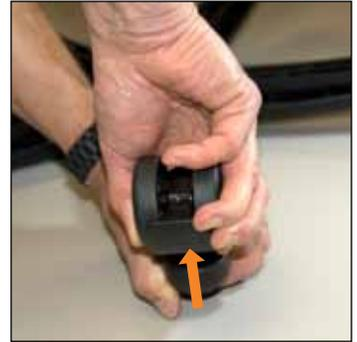
4. Grasp base with one hand (gloves suggested) and pull caster out with the other. Repeat on each leg. If any are stuck, you can pry it out using a flat screwdriver.
