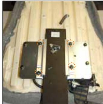
6. Remove four 3/8" Allen heads bolts securing the aluminum sleeve to the pressure plate.
