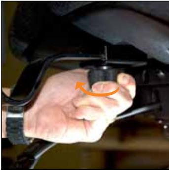
1. Loosen and remove the handwheel which secures the arm in the bracket under the seat. Keep washers in same order for reinstallation.
