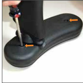
3. Turn the arm upside down and remove the 2 Phillips head screws (standard pads) or 3/16" Allen head (OES pads). NOTE: Arm pad must be rotated 90° to allow access to the rear screw.
