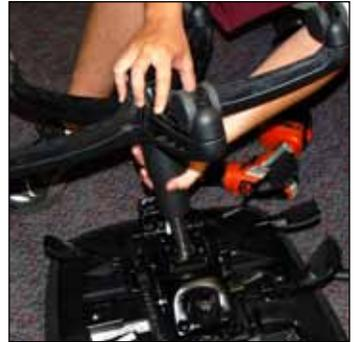
8. Replace the cylinder and base assembly by placing the cylinder into the mechanism and pressing firmly.
