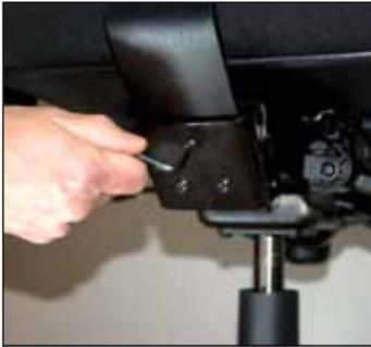
1. Remove the 3 screws (3/16" Allen wrench) that secure backrest post to the mechanism. Once detached, place on a clean work surface with the outer shell up and accessible.
