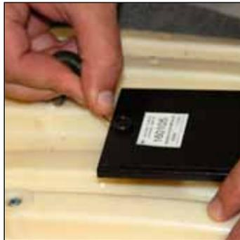
6. Stretch spring to reach keeper on the JBU and slide over head.
