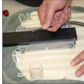
3. Start the four 5/32" Allen-head screws and tighten to secure the new headrest bar to the internal height adjuster.
