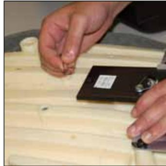
3. Slip the lower spring from the retainer on the JBU (i.e. back post).
