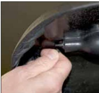
5. Attach the lumbar pillow air hose to the nipple of the bulb reinstalled in step 4.
