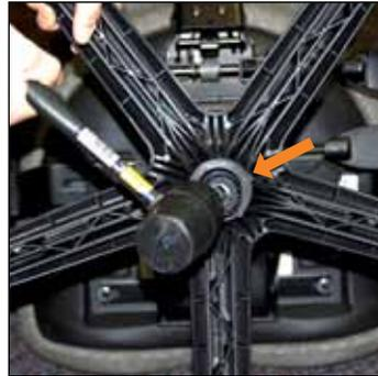
2. Using a plastic hammer, strike the bottom of the cylinder while firmly holding one leg of the base to dislodge the base from the cylinder.\*
