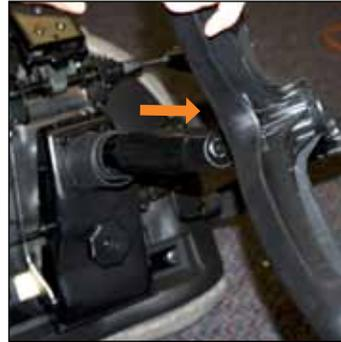
3. Remove the base completely from the cylinder.
