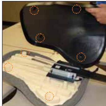
6. Position and install the new back shell by aligning the tabs with receiving bosses.
