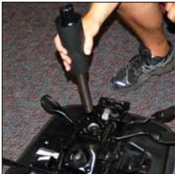
5. With cylinder out of the mechanism, slide the cover off. You may reinstall the old cover on new cylinder, or use new cover (Step 6).
